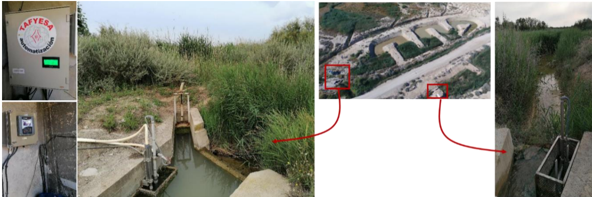
Figure 8. Gauging stations (inlet and outlet), automatic sensors and controllers for telematic measurements at the CW facilities
