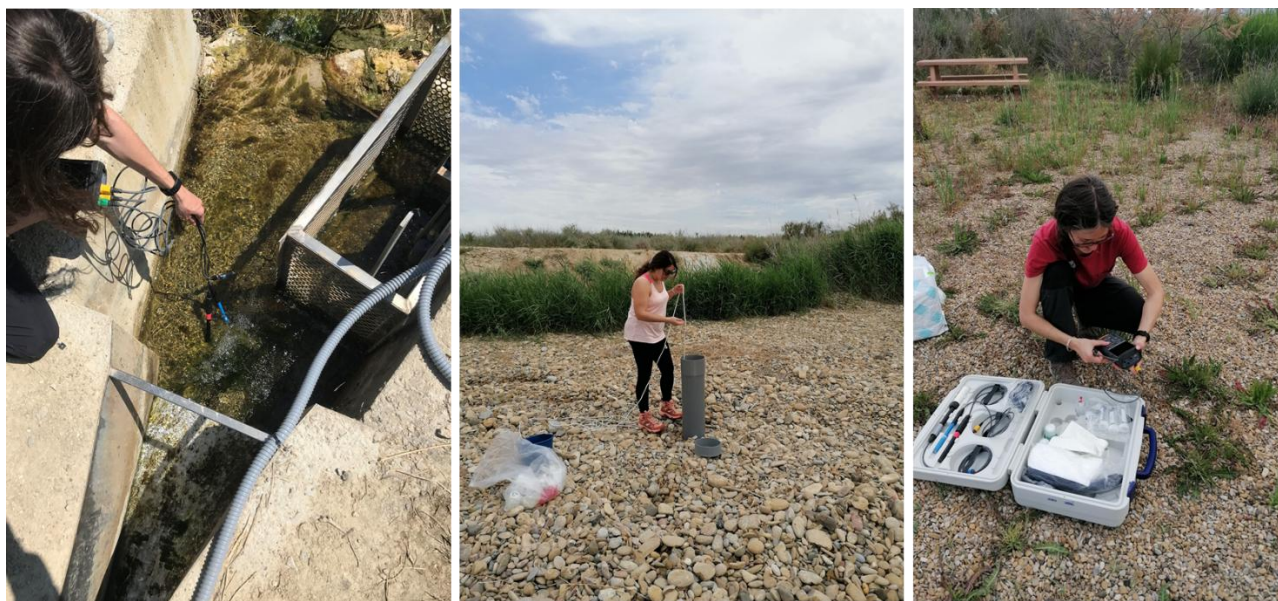
Figure 9. Measurement of parameters, water sampling and preparation of samples before analysis at the CW facilities
